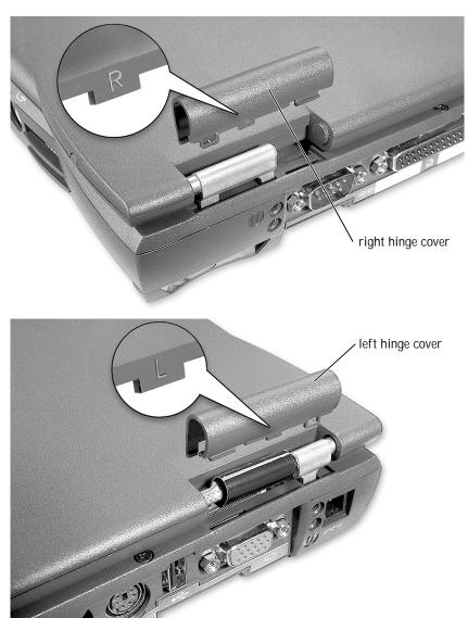
1 Attach the display assembly to the bottom case assembly.
