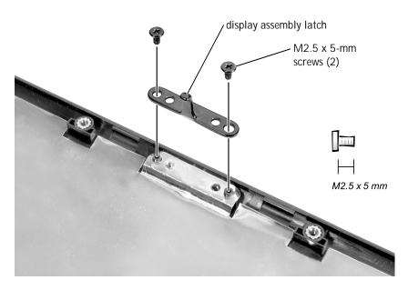
Removing the Display Assembly Latch
