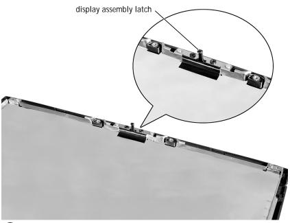
NOTICE: Do not remove the display assembly latch from 14.1-inch SXGA+ and 12.1-inch display panels. If the latch is damaged, replace the display-assembly top cover.
